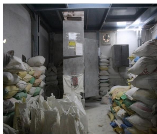
Magnet Separation Area – to remove free iron particles from raw material
