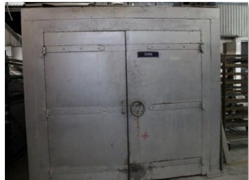
Gas oven – the bricks are dried in our gas oven before going for firing to remove the moisture
