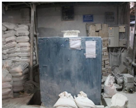
Ball mill-2 – for crushing raw material into fine powder
