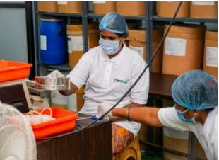
Seaving of raw material particles taking place through seaving machine
